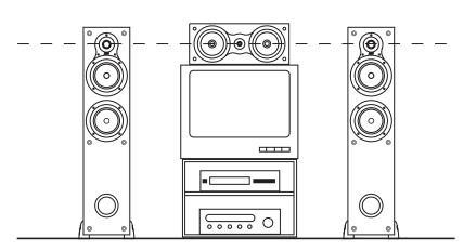
Figure 3 Proper Placement of Center Channel Speaker
